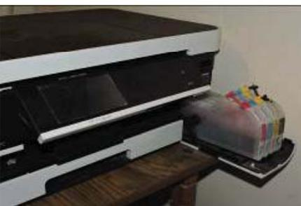
I have had a CIS for my Brother printer for nearly two years and after the initial slightly awkward installation the system has been running just fine. This system uses extra large cartridges that extend out of the ink cartridge compartment, beyond the front of the printer and have refill openings (plugged) on the top, which are reasonably easy to access. The car-
